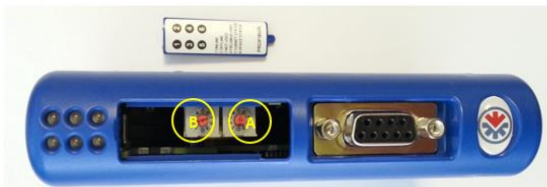
Figure 13 - Profibus module switch identification
