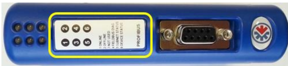
Figure 12 - Profibus module switch location
