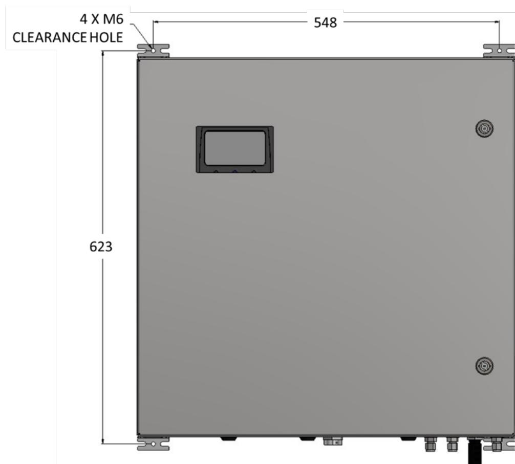
*Figure 4 - BIOGAS 3000 enclosure dimensions*
