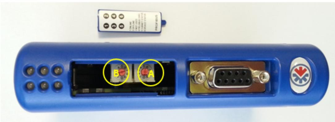
Figure 9 - Profibus module switch identification
