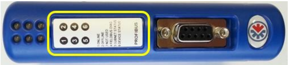
Figure 10 - Profibus module switch location
