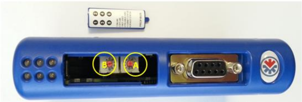
Figure 11 - Profibus module switch identification
