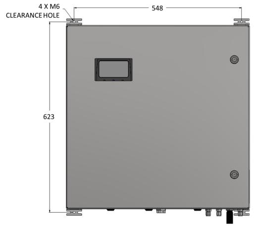
Figure 4 - BIOGAS 3000 enclosure dimensions
