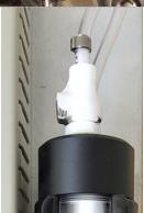
Once secure, reconnect the couplings to the catchpot top, ensuring the tubing is not trapped or kinked.
