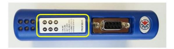
Figure 8 - Profibus module switch location
