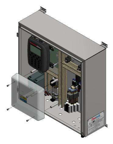
Figure 6 - Mains cover removal
