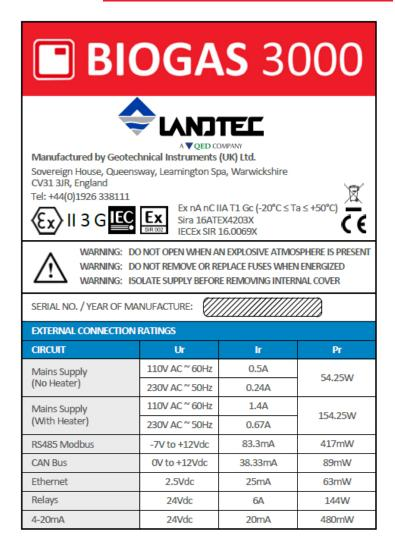
Figure 7 - BIOGAS 3000 electrical label
