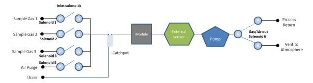
• The BG3K3 also has the option of measuring from the hydrolysis tank on sample point 1 and not passing this gas across the external sensor. This prolongs the life of the sensor. The following image is a block diagram if the system with this option selected:
