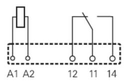
Wiring Diagram 4 - Relays
