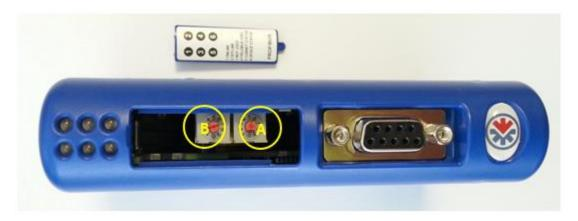
Figure 9 - Profibus module switch identification
