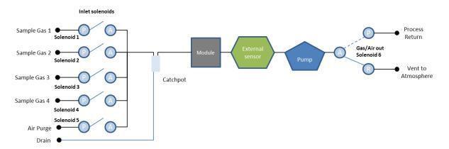
The BG3K4 also has the option of measuring from the hydrolysis tank on sample point 1 and not passing this gas across the external sensor. This prolongs the life of the sensor. The following image is a block diagram if the system with this option selected:
