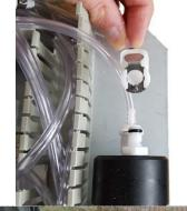
Disconnect the QRC from the top of the catchpot.
