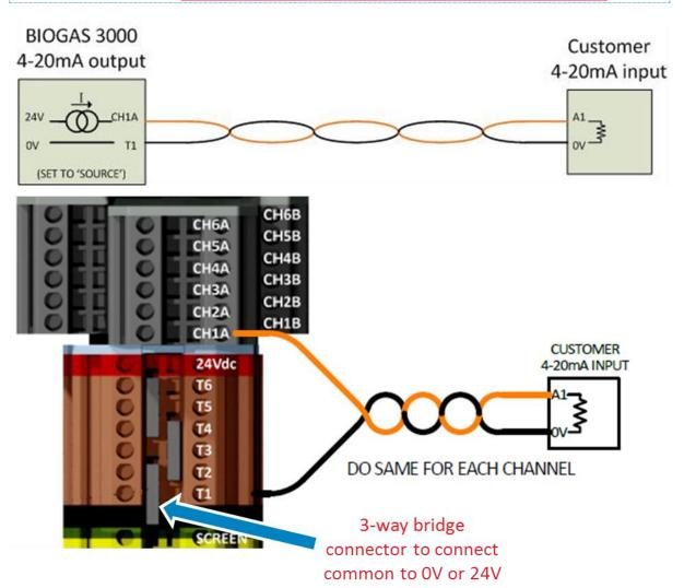
Wiring Diagram 3 - 4-20mA circuit
