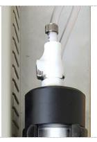
Reconnect the system tubing by connecting the QRC to the top of the catchpot.
