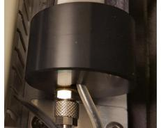
Gently position the catchpot so that the drain tube is closest to the backplate and the female QRC is facing the front.
