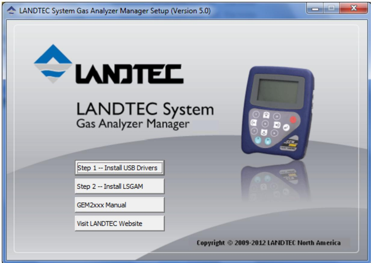
The instrument communicates to the computer by means of a USB. This USB cable requires drivers to be installed prior to use on the computer. From the CD (or USB memory stick) choose the first option “Step 1— Install USB Drivers”
