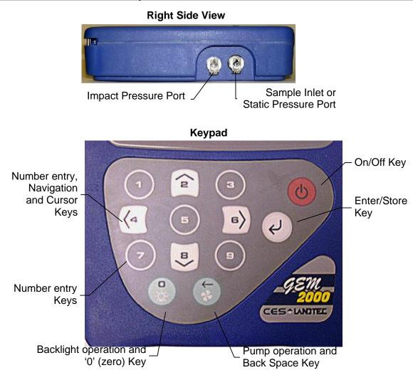
Whenever a key is pressed the unit will emit a short 'beep' as an acknowledgement. This function cannot be turned off.
